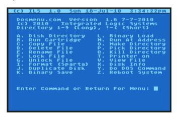
If the [R] option is chosen, the DOSMENU will be made resident in memory. Now it is possible to leave the menu by pressing <B> to BASIC and write e.g. a program. After finishing the BASIC task you will get back to the DOSMENU by typing **DOS<RETURN>**.
