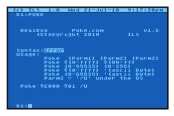
POKE allows you to change memory locations from the command processor, which can be useful in batch files and other applications. It is very easy to crash the system with it, if you do not really know what you are doing. Some examples of POKE locations and useful values:
