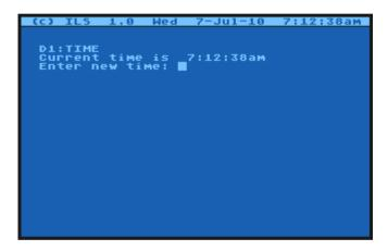
**Note:** An easy way to update to the current time/date is to use TDLINE2.COM with a SIO2PC or APE Interface and APE software or AspeQt on the PC.
